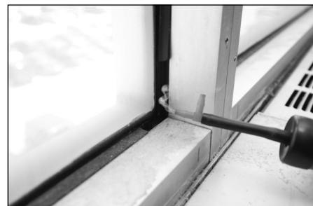
blower door test or thermal imaging, to pinpoint exactly where air is entering the building. The air leakage detector is a hand-held device that emits smoke when squeezed. It works by visually showing how air is moving in the space – where the smoke moves, air is
